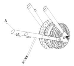
5. Install a 4mm bushing **(A)** and an M12 cap nut **(B)** onto the motor axle from each side, and tighten them.
