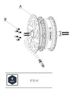
2. Install the freewheel (A) onto the motor axle from the right side, and tighten it.
